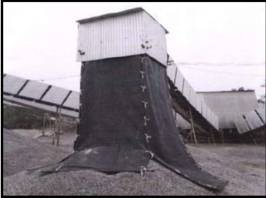
Figure-2: Chute from top of discharge point
